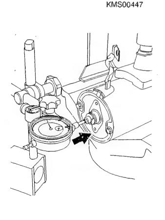
Checking and adjusting armature axial clearance
